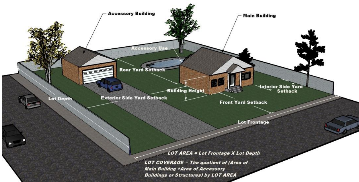
Figure 2.4: Main Building and Accessory Building
